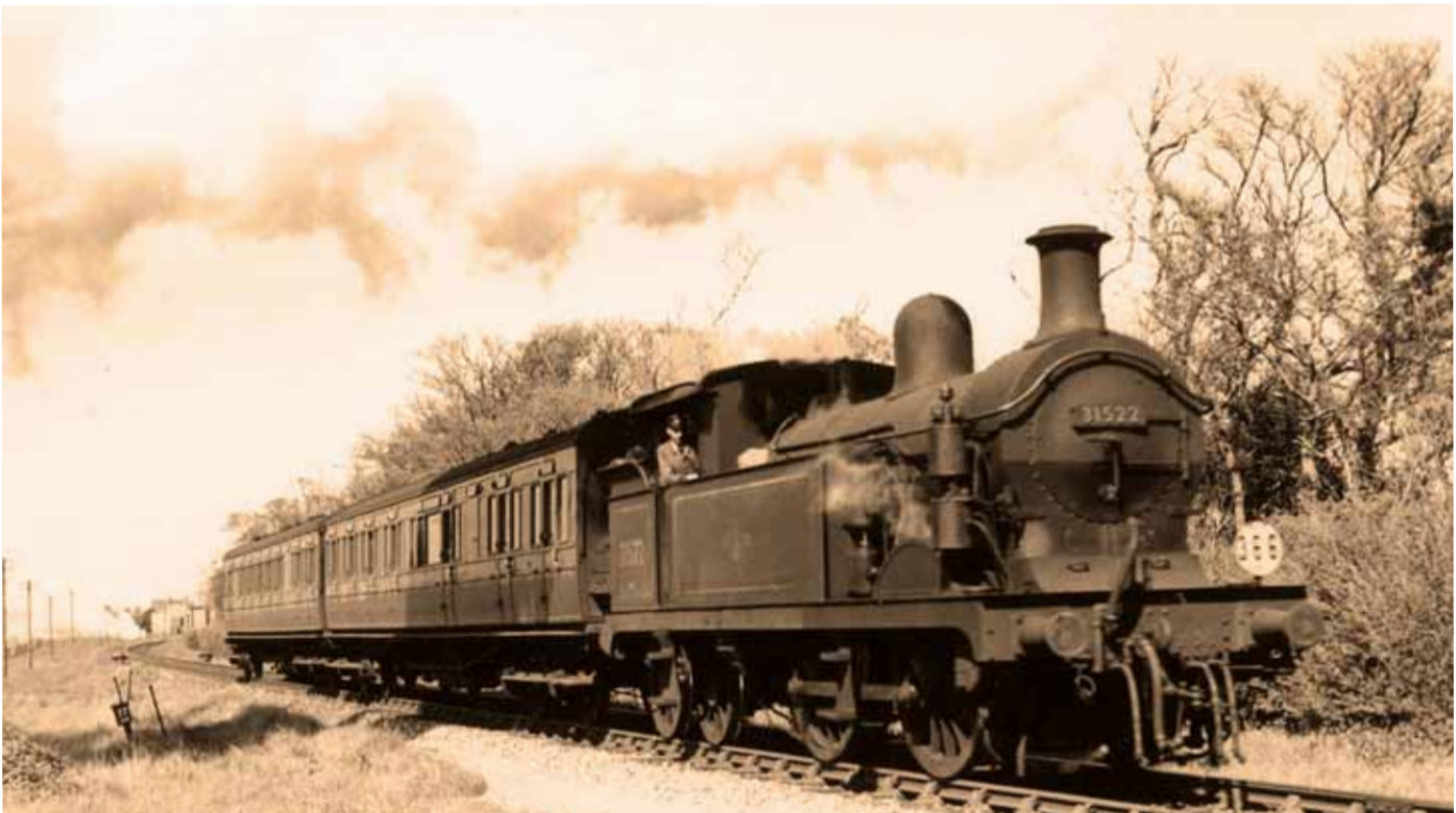
The New Romney Branch / Southern Railway, approaching Church Lane crossing. Engine: one of the faithful Class H 0-4-4 tanks. She would be around 55 years old when the photo was taken.
