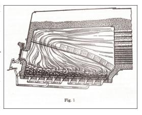
Most of the coal from the Eastern States is of the harder varieties, so that it has a lower percentage of slack and a higher percentage of lumps, many of which are too large to go through the firedoor. Now, fine coal and large lumps cannot be burned together, because the lumps burn slowly and tend to cause banks and clinkers; also, holes form around the lumps. A fireman will save worry and labor by breaking up large lumps to the size of medium-sized apples before shoveling them into the firebox.
