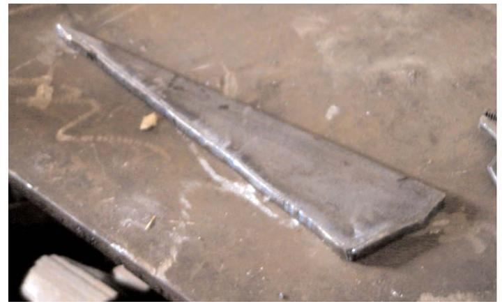
flat bar, I could grind the weld to mimic the rounded edge of the rail. This was probably the most complicated part of the operation. Note: the wide end of the cap is cut to match the angle of the rail.
