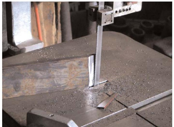
Next part is to cut the base plate for the frog and lay it out, and weld it into place. I used 3/8" plate,
