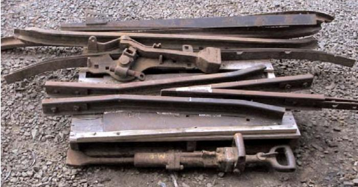
My first step was to bend the long rail. Since I was using short rem's they were already drilled for joiners and I didn't have to do that operation, but that will happen on the next ones. I'll pre drill before I bend. After I made my bends, I cut the rail to length. I did that because of the size of my rail bender. It is the old Jim Crow type modified with a hydraulic jack. The
