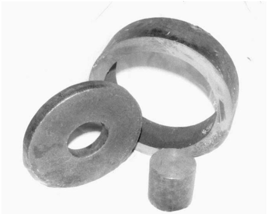
the lathe and prepare the “doughnuts” for welding. “What?” you say, “can’t I just stick ‘em together?” NOPE. Both the outside and inside diameters of the doughnut need to be beveled on both sides to allow a complete weld at the joints. Thus the 3 pieces become a homogeneous whole.
