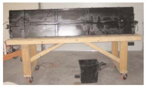
or locomotive on the wood car stand because I built the top from plywood. I have to tip the car over on my wood stand to work on the bottom, but that is an advantage once the car is over on its side because I am working standing up.
