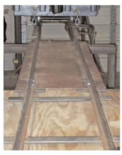
holds the car (or locomotive). There is a hole in both where a bolt is placed, and nut tightened. Now the car (or locomotive) can ride smoothly from truck to car stand and the four foot plate cannot move and does not flex badly under my locomotive, and not at all under my flat cars.
