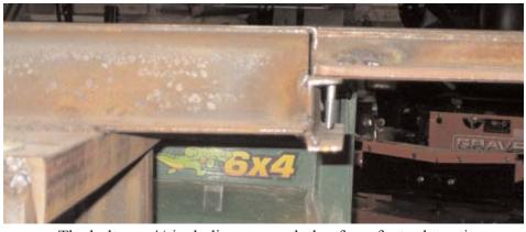
The bolts are ¼ inch diameter and about 2 inches long. There are no nuts. The car stop lifts off when needed. This is not a great system since the car rolls back and forth from end to end. I now use a clamp on the channel iron, clamped right against the wheel as shown below.
