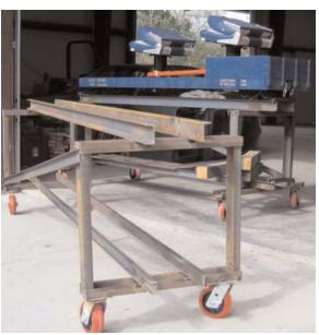
give it better support side to side. A locomotive weighs more than a car, so I felt that it should be wider to be more stable. My loco weighs 1405 pounds, so I am happy to have the wider stand. My flat cars weigh 300 pounds and the 27 inch wide cross pieces are rock solid with this weight or even with one on top and one below.
